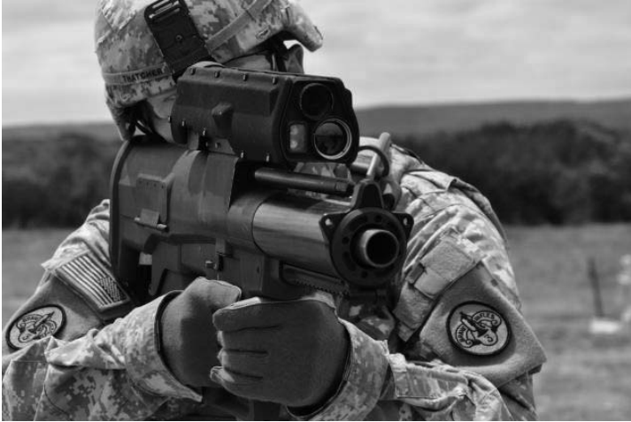
XM25 shoulder fired, semi-automatic 25 mm grenade launcher
